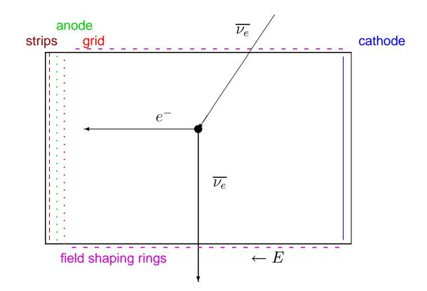
The TPC is an acrylic chamber, diameter 90 cm, length 160 cm filled with 3 bar CF4 gas.
