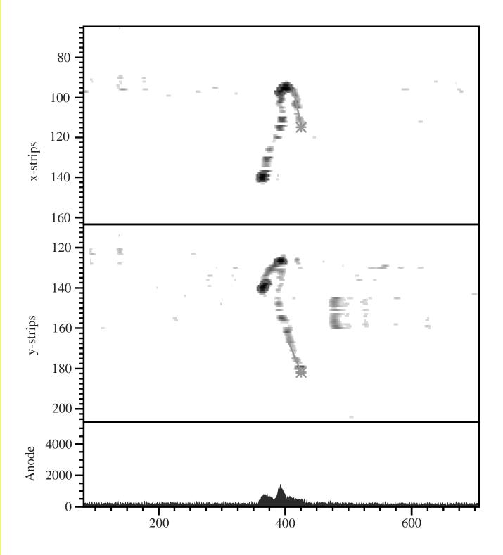
An electron of 925 keV with direction fit and vertex
