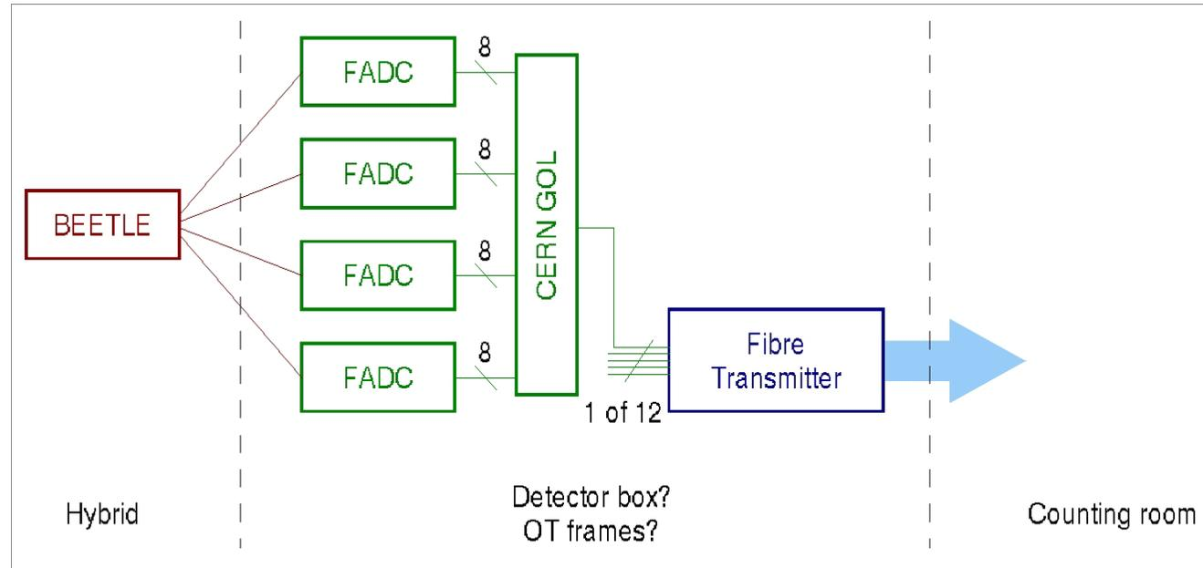
digital optical readout link at 1MHz
