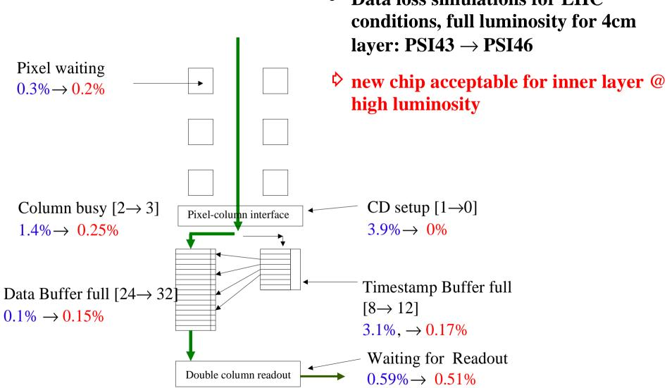
Data loss simulations for LHC conditions, full luminosity for 4cm
