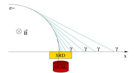
\* Earth magnetic field taken as bending magnet for e<sup>±</sup>> some 500 GeV
